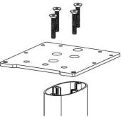
3. Assemble foot to leg extrusion with four (4)  $\frac{4}{20}$  x 1.5" flat head cap screws and push casters into feet if applicable.
